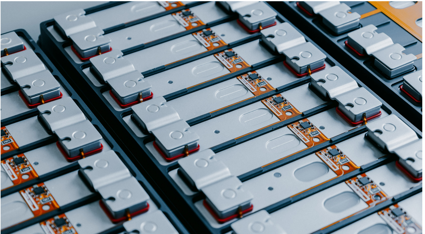
Prismatic cells equipped with Dukosi Cell Monitors
