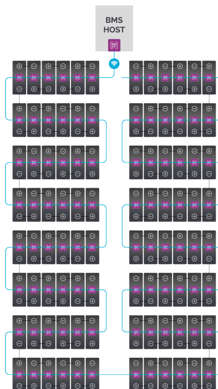
Figure 4: Near field contactless BMS design using Dukosi DKCMS connected to a 3 rd party BMS host
